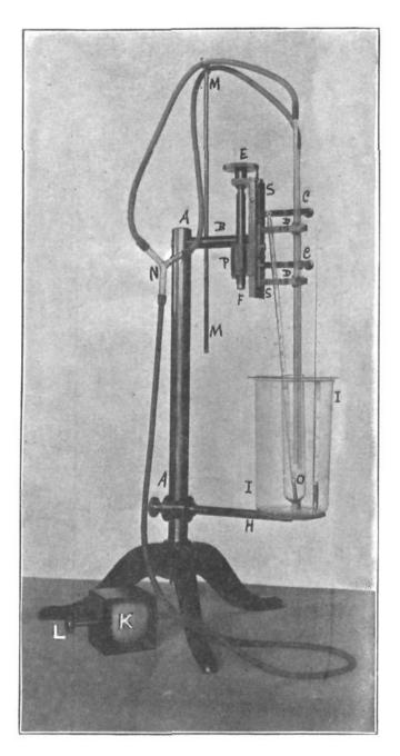
Fig. 1. Apparatus for Determining the Surface Tensions of Liquids. (To Face p. 516.)
